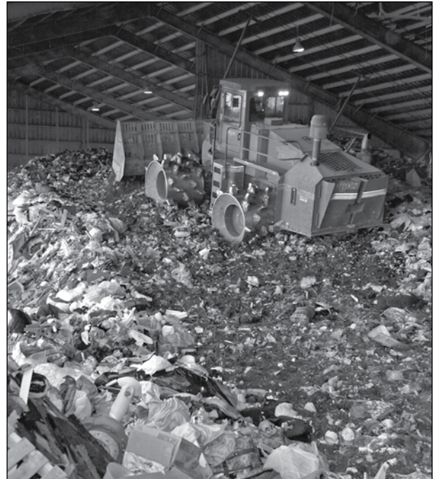
The trash compactor in full operation at the Ley Creek Transfer Station in Liverpool. Compacting C&D material minimizes the number of loads OCRRA hauls for final disposal, which minimizes greenhouse gas emissions.
