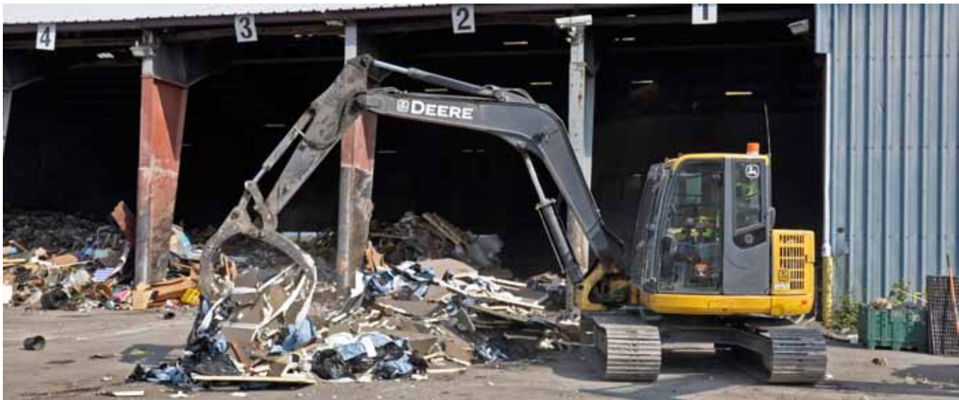
Ley Creek Transfer Station staff uses an excavator to separate recyclable material (e.g., cardboard and metal) from the trash.
