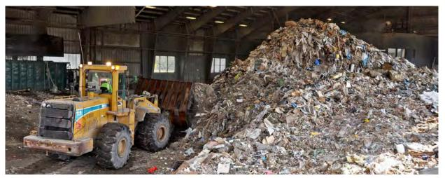
A large wheel loader operator amasses trash at the Ley Creek Transfer Station before depositing it in a trailer for delivery to the Waste-to-Energy Facility in Jamesville, NY.
