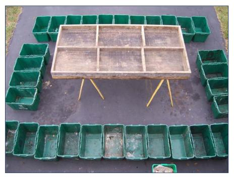
Figure 2-3 Typical Manual Sorting Layout
